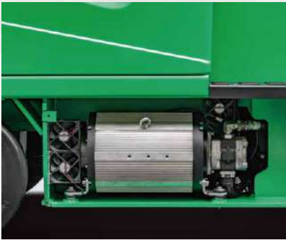
The EE rated forklift's electrical components are enclosed to prevent sparks in hazardous conditions.
