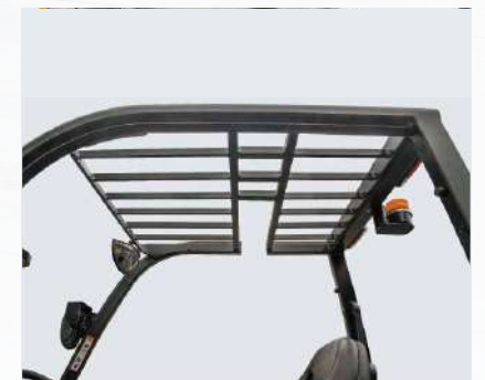
The strong overhead guard exceeds ANSI and ITSDF regulations and offers great protection while maintaining excellent all-around visibility.
