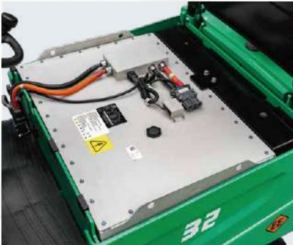
The EE rated forklift features a sealed Lithium Iron Phosphate (LiFePO 4 ) battery pack.
