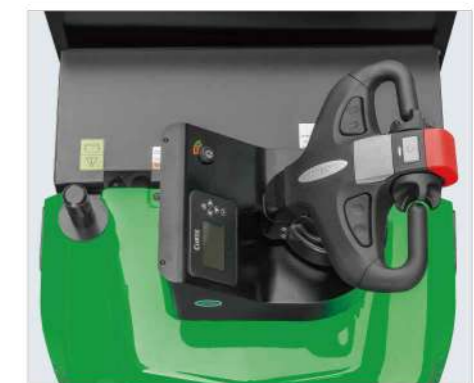
The tiller and instrument display can be moved sideways to allow for more room when changing the battery.
