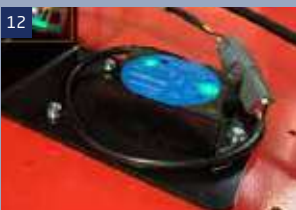
Angle sensor: when it is lifting and walking on the slope, the sensor will automatically judge the status of the machine, if the angle is larger than the rated angle, it will alarm to remind the operator.
